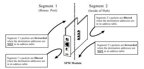
Figure 2.5b: Forwarding vs. Filtering in SPM Modules
